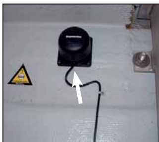
AUTOMATIC PILOT COMPASS
