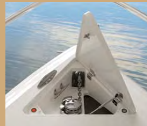
Fresh water washdown in windlass compartment.
