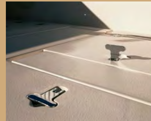
Custom Intrepid T-handles secure gasketed hatches that remain silent.
